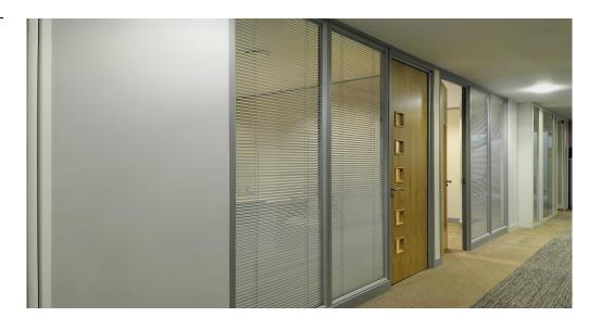
Similar to Komfire, Kameo is Komfort's 75mm distinct radiused style steel stud and plasterboard construction, surrounded by an aluminium framework. This system incorporates acoustic performance of up to 43dB (Rw) and fire protection of up to 30/0 for the glazed system.
