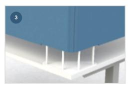
Lower the panel onto the 4 spigots in both corners.
